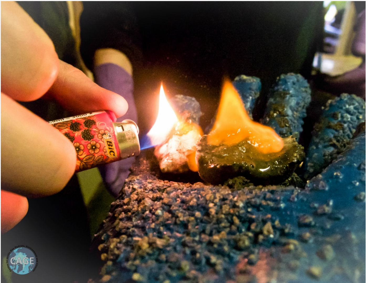
Gas hydrate is also known as the ice that burns. You can literally set it on fire. It is a solid form of gas, often methane, which is maintained in great depths or under high temperatures. Photo: CAGE
